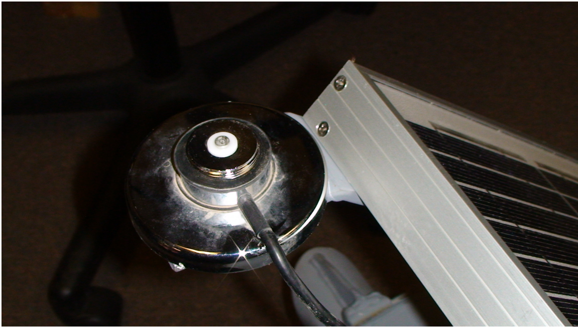
Photo 2. Antenna base on top of the solar bracket.
