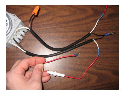
The photo above shows the timer power portion of the wiring harness. The Red cable with terminal ring and the 1 amp fuse holder is connected to the (+) positive battery terminal. The black wire with the terminal ring is attached to the battery (-) negative terminal.
