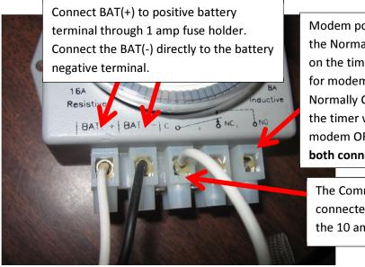
Modem power (+) wire connects to the Normally Open (NO) connection on the timer when setting the timer for modem ON times. Connect to the Normally Closed (NC) connection on the timer when setting the timer for modem OFF times. **Use either but not both connections.**
