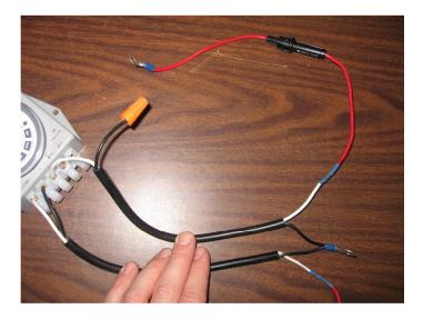
Photo above shows the load portion of the wiring harness. The Modem power cable (-) negative side is connected to the battery negative side at the orange wirenut. The Red cable with terminal ring and the 10 amp fuse holder is connected to the (+) positive battery terminal. The black wire with the terminal ring is attached to the battery (-) negative terminal.
